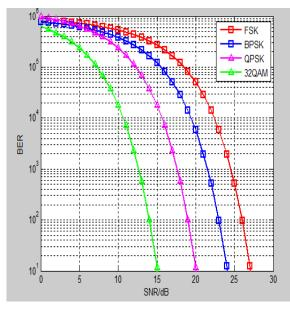
Fig. 4. Analysis of PLCC- FSK 26 SNR/db, BPSK, 24 SNR/db and QPSK 20 SNR/dB with 32QAM 15 SNR/db proposed.
