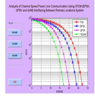
Fig. 3. Analysis of PLCC- FSK 26 SNR/db, BPSK, 24 SNR/db and QPSK 20 SNR/dB with 16QAM 16 SNR/db proposed.
